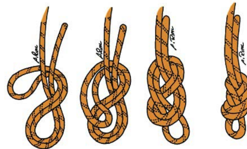
Figure of 8 laid
