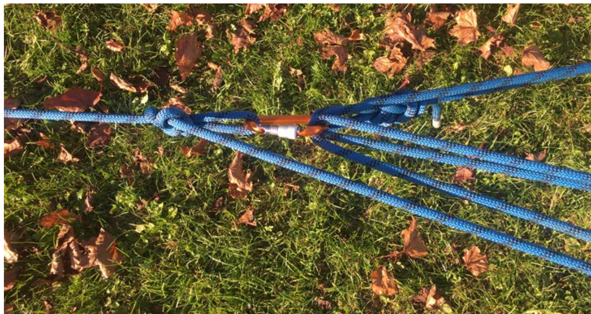
Fig. 9.7: Load distributing "Boatman's" 3 point Anchor using main line (close up)
