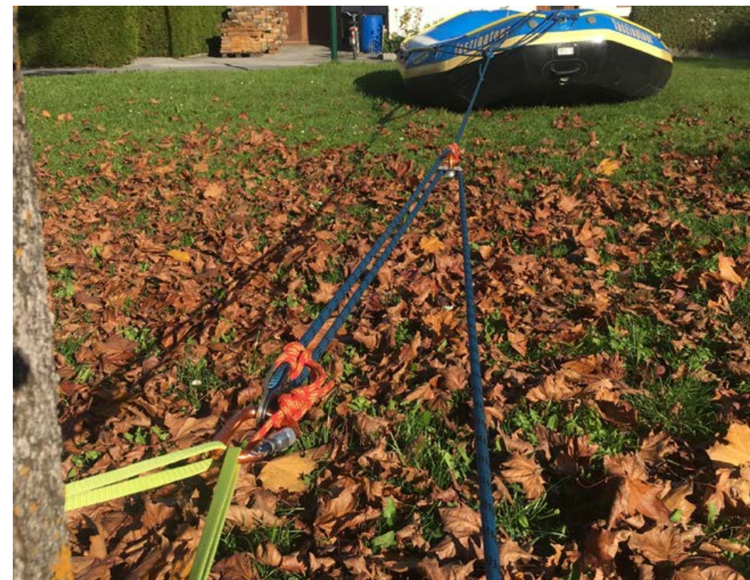
Fig. 9.9: Overview Z-drag using Static line for both the main line and anchor
