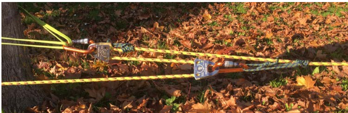
Fig. 9.3: Basic Z-Drag using throw bag and 2 pulleys
