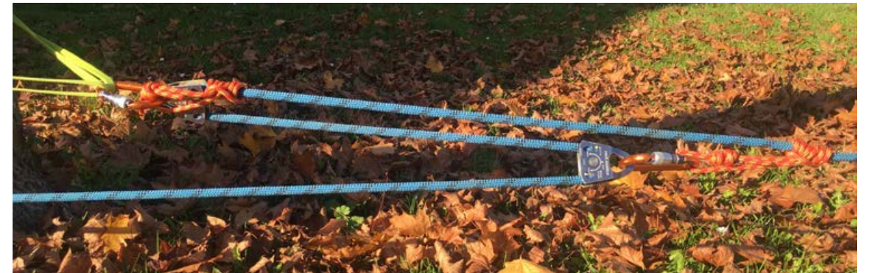
Fig. 9.4: Basic Z-Drag using 11mm static rope and 2 pulleys
